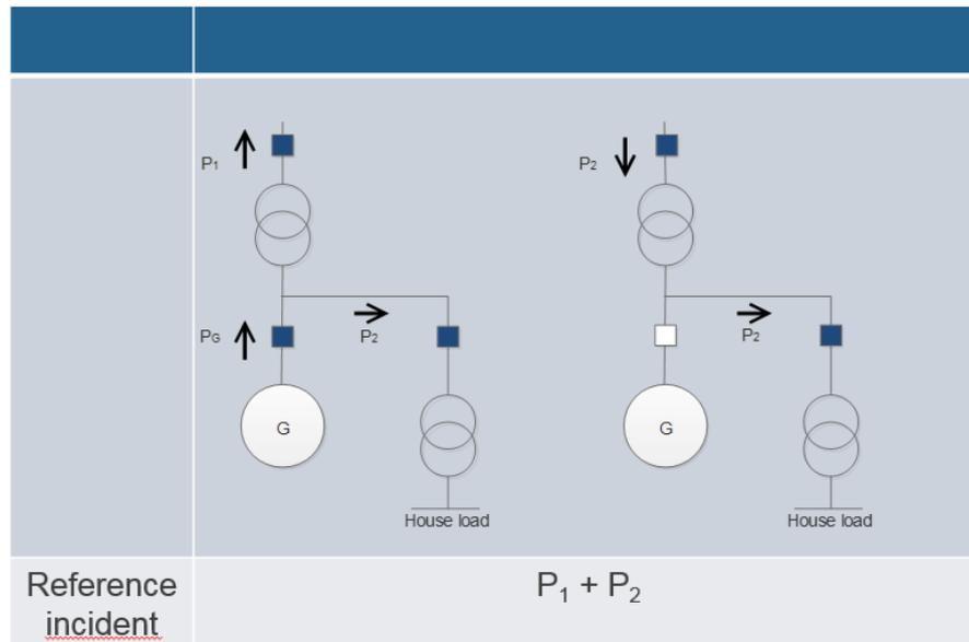
Figure 2: The 'incident considered' is the actual change of power after the trip of a generator unit. The house load shall be taken into account. 'Reference incident' equals the sum of  $P_1 + P_2 (= P_G)$
