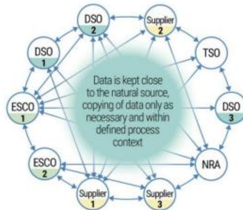
Figure 1: Schematic representation of data model in a decentralised environment 6,7
