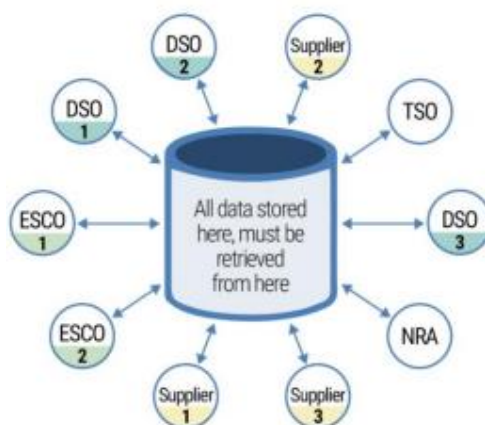
Figure 2: Schematic representation of data model in a centralised environment 6,7
